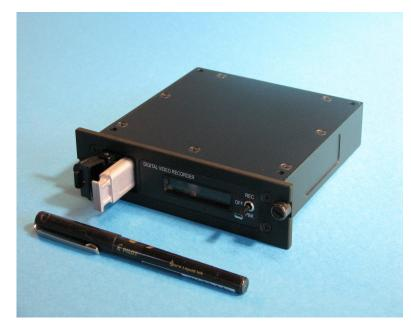
The use of a rugged "disk-on-key" as the recording media provides a low power, light weight solution for applications requiring low-cost reliable data storage.
